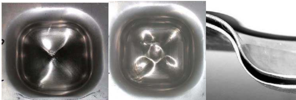
Fig. 16. Deformed steel obtained with the CNC machine.
