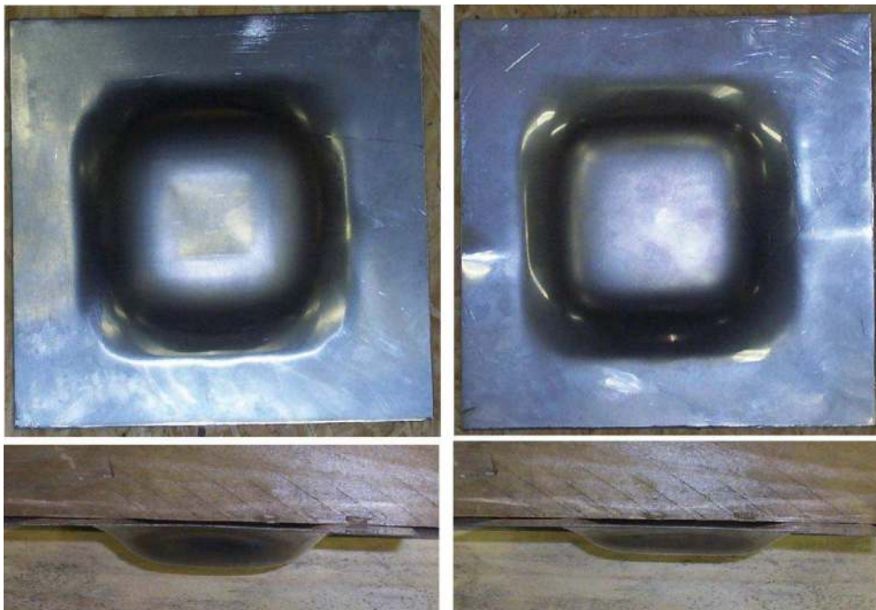
Fig. 15. Deformed steel parts for direct (left) and inverse (right) forming obtained with the robotized cell.
