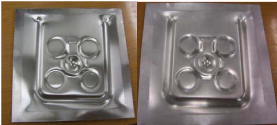
Fig. 18. Formed chair backs: AISI 304 (left) and DC04 (right).
