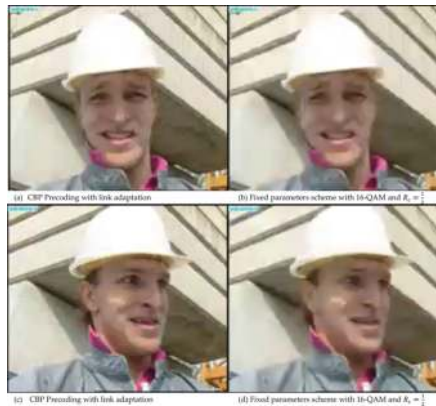
Figure 9. Example of reconstructed frames for Foreman video for CBP precoding with link adaptation ((a) and (c)) compared to a static scheme with 16-QAM modulation and rate 1/2 channel code ((b) and (d)).
