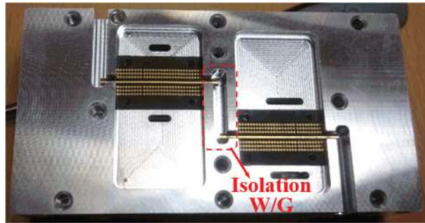
Figure 4. Fabricated transitions and assembled in the metal case.
