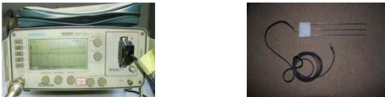
Fig. 1. Left: The frontal panel of the Tektronix 1502B reflectometer with rise time t_r = 0.3 ns. Right: A three arms probe.
