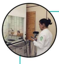
Epirradiator test (250 – 350 °C) The burnings that exceeded 60 seconds: classified as "negative burning".
