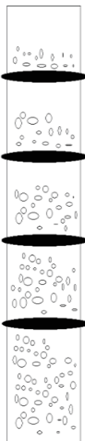
Fig. 2. The situation of gas-liquid mixture in the simulation test of desulfurization tower
