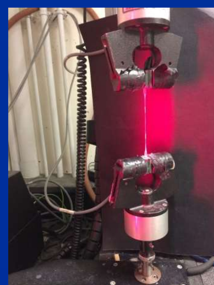
Figure 1: Tensile test, showing Instron grips and red light from optical extensometer
