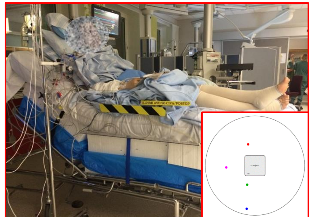
The custom made bed with 1' of Styrofoam lifting the mattress with EM generator from the magnetic bedframe. Insert shows the positions of the EM sensors in AP projection: blue – pressure sensor, red & green – lateral sensors, magenta – sensor in CVC.
