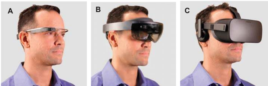
Figure 1. Head-worn Computers or Displays Vary in Size, Weight, and Face-Obstruction. (A) Glass Explorer Edition (originally known as Google Glass): AR smartglasses with a fully stand-alone onboard computer (weight 42 grams). (B) Microsoft HoloLens: AR headset with a fully stand-alone onboard computer and depth camera (weight 579 grams). (C) Oculus Rift: VR headset display, which must be tethered continuously to a powerful computer to drive it (weight 470 grams). VR headsets and some AR devices are large, heavy, and block the social world considerably. Image depicts the study author, NTS.
