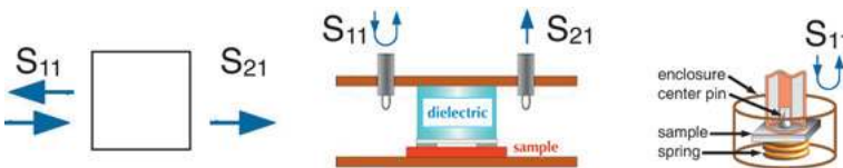
Fig. 8.4: (a) Sketch of a generic two-port device, containing the superconducting sample under investigation; (b) a typical dielectric resonator setup; (c) a typical Corbino disk setup.
