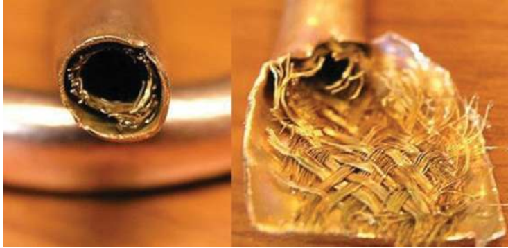
Figure 4. Screen mesh wick [15].
