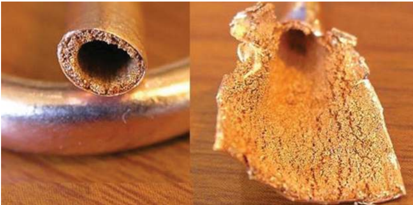
Figure 2. Metal sintered powder wick [15].
