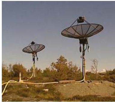
Figure 1. The 2.3 m radio telescopes of the Onsala Space Observatory.
