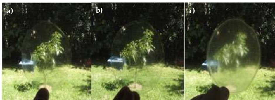
Fig. 1a. Film of CS + CNC (0.5%). 1b. Film of CS + CNC (1.0%) and 1c. Film of CS + CNC (2.0%)
