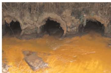
Figure 1. Acid mine drainage associated with gold mining in the Krugersdorp area (As is about 6150 µg/L).
