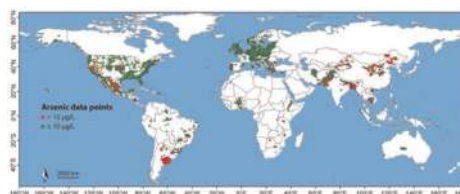
Figure 1. Arsenic concentration measurements excluding those known to originate from a depth greater than 100 m, averaged to 1-km square pixels (n = 58,555).
