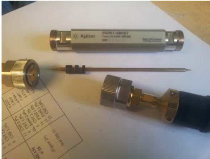
Figure 2. Coaxial airline 50 \Omega probe used for the dielectric characterization of nanocomposite materials and for the measurement of EM reflection and transmission properties of layered materials.
