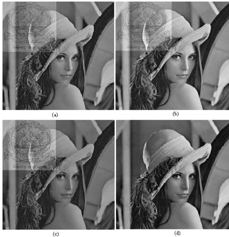
Fig. 8. The images obtained after watermarking (a) for \alpha=0.97 and \beta=0.07 (b) for \alpha=0.97 and \beta=0.17 (c) for \alpha=0.97 and \beta=0.27 (d) invisible watermarking
