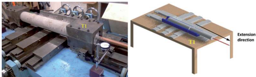
Figure 4. Instrumentation of extension bench test (adapted from [18]).
