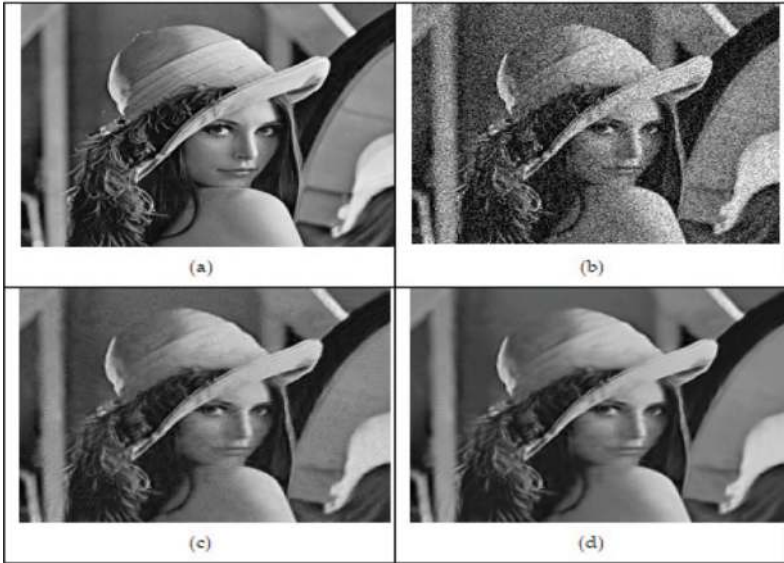
Figure 14. (a) Clean image (Lena.tif), (b) Noisy image with, (c) The denoised image by the proposed technique (the first stage) and denoised image by the proposed technique (the second stage).
