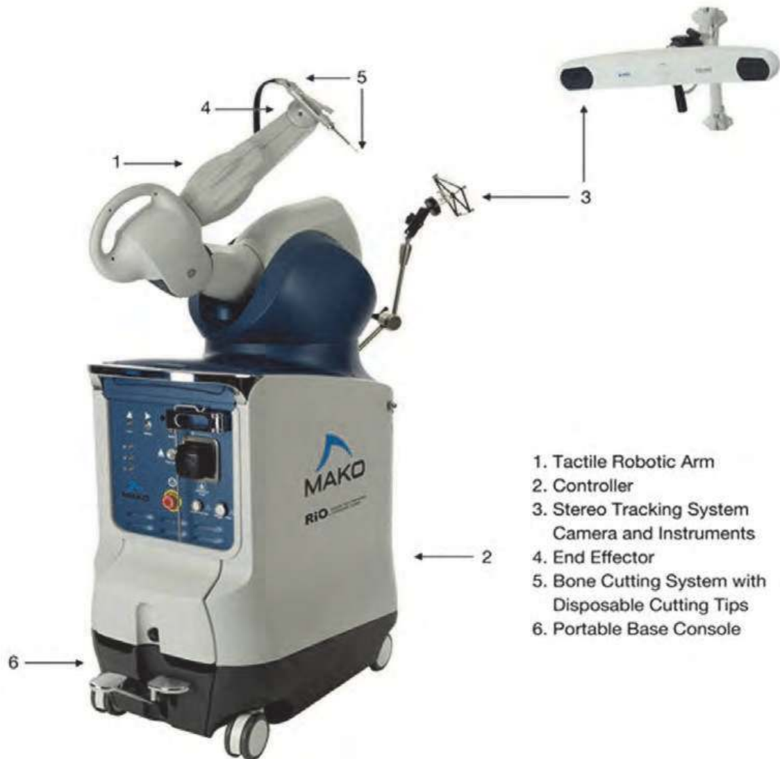
Fig. 10. MAKO Tactile Guidance System (TGS) (MAKO Surgical Corp., Fort Lauderdale, Fla)
