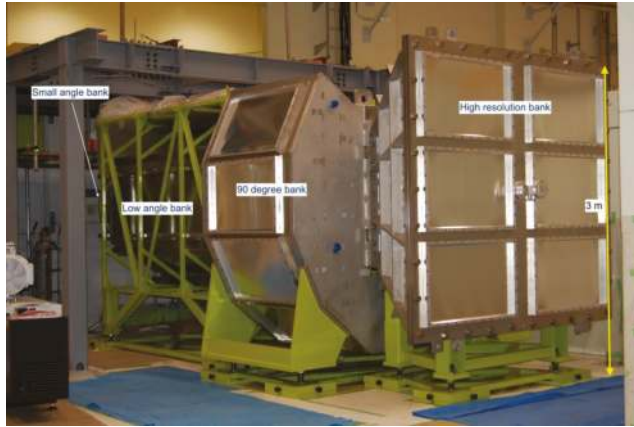
Figure 17. IBARAKI Materials Design Diffractometer, iMATERIA without detector for each bank and instrument shielding. The high-resolution bank, special-environment bank (90° bank), and low-angle bank, can be seen from right to left. The small-angle detector bank, which is not shown in the picture, is situated in the low-angle vacuum chamber (left hand side of the picture).
