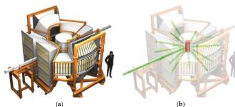
Figure 14. (a) Overview of SPICA instrument. The horizontal detector crates are arranged on a cylindrical locus from 2\theta = 5^\circ to 175^\circ . (b) Illustration of operando measurements. An 18650-type cell is placed at the center of the sample chamber. The neutron incident beam enters the sample chamber, where it is diffracted by the electrodes, and subsequently reaches the detectors.
