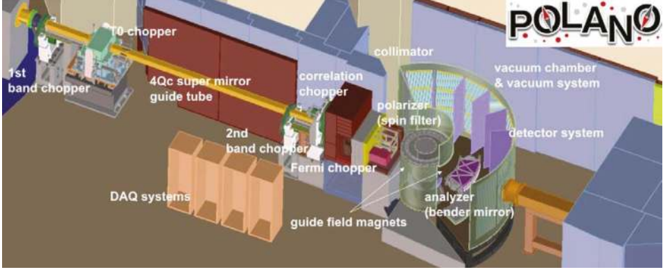
Figure 8. Schematic POLANO beamline and instruments. Neutron beam coming from left-hand side is injected into vacuum chamber (sample) [38].
