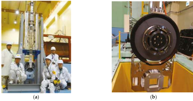
Figure 4. Pictures of (a) the rotating muon target assembly; and (b) the rotating muon target itself.
