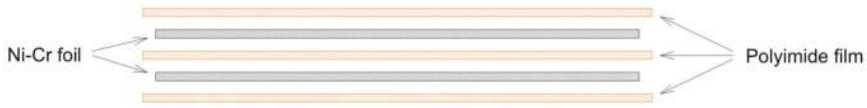
Figure 11. The structure of non-magnetic flexible heater. Two layers of Ni-Cr foil are sandwiched between a polyimide film for electrical insulation. The overall thickness of the heater is less than 0.5 mm.
