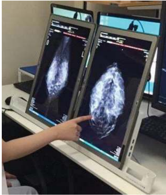
Figure 2. Two sets of 4K tablet PCs with high-resolution color monitors (4K UT-MA6, 2560 × 3840 pixels, 20.8 inch; Panasonic).
