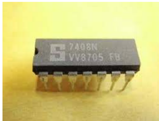
Figure 4-7: 7408 chip, notch indicates top of chip.
