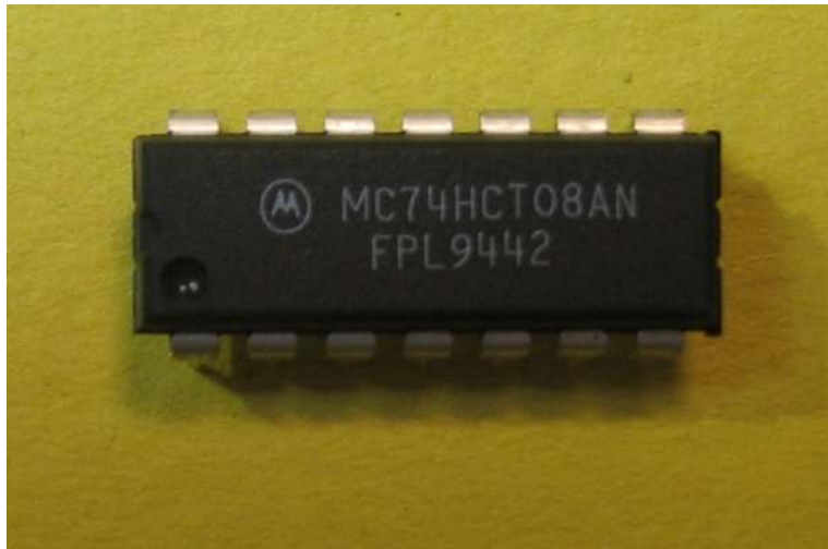
Figure 4-6: 7408 chip, circle indicates top of chip.
