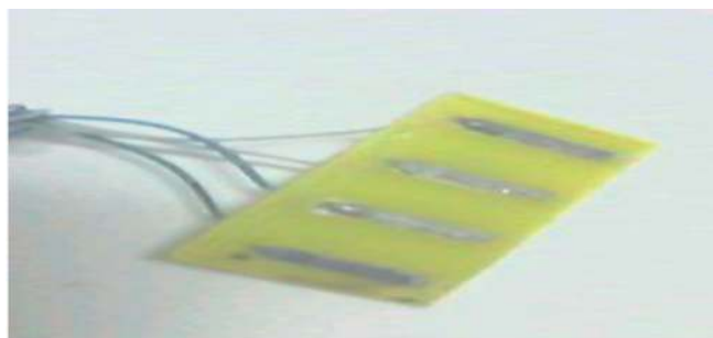
Figure 5. Four-electrode probe for measuring electrical conductivity.
