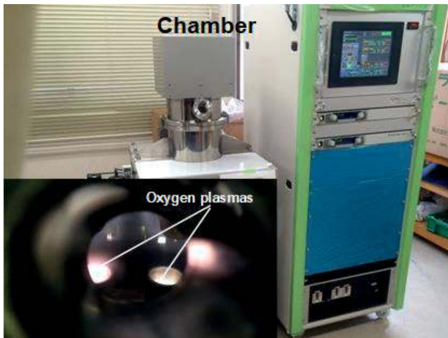
Figure 21. Simultaneous ashing system of two diamond-coated cutting tools toward industrial demonstration.
