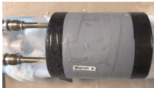
Figure 9. A quadrature birdcage RF coil for mice (Morris instruments, Ottawa, ON): 97.3 MHz, 3 cm in diameter and 6 cm in length, was used for used for high-resolution ^3\text{He} imaging.
