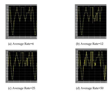
**Figure 12.** Received signals with different rate of interference
