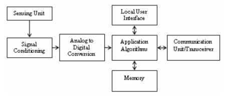
Figure 1. Basic architectural components of a smart sensor
