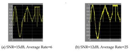
Figure 7. Received signals with different rate of interference & different SNR
