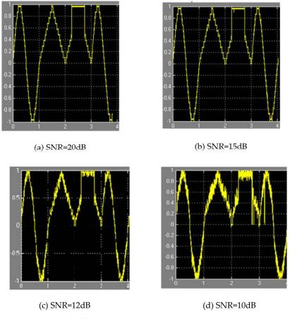
Figure 4. Received signals with different SNR
