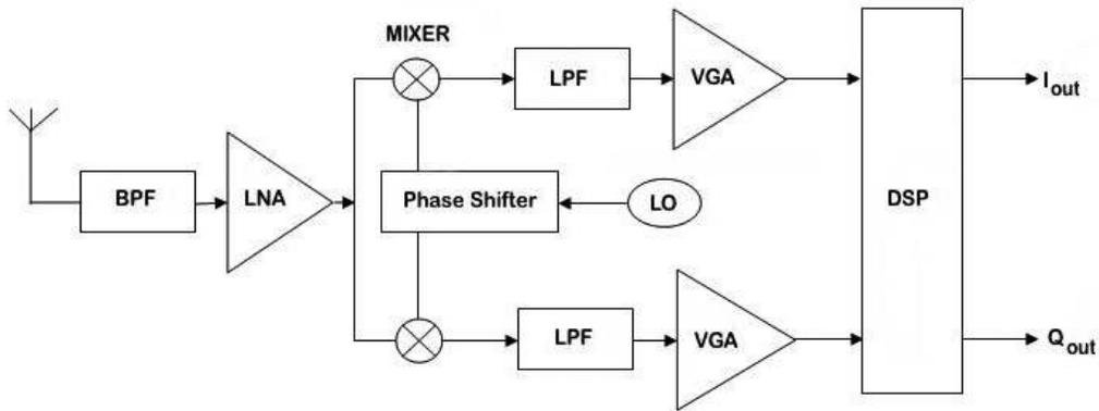
**Figure 1.** Direct conversion receiver.
