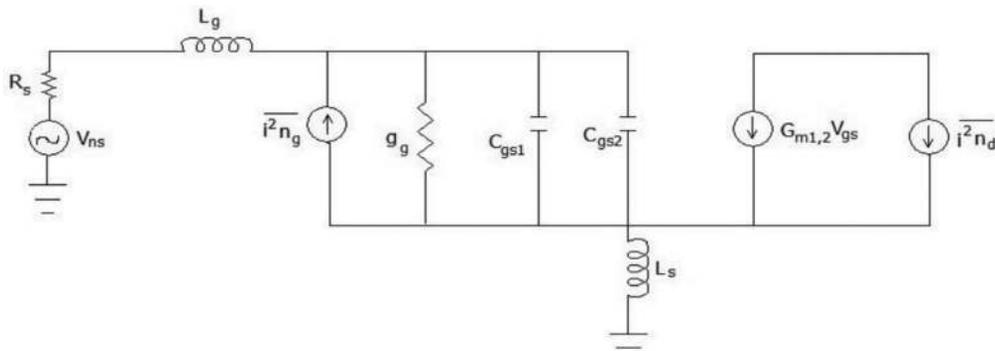
**Figure 13.** Equivalent noise model of input stage.
