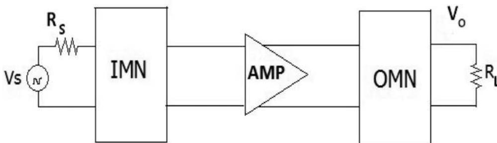
**Figure 6.** Block diagram of LNA.
