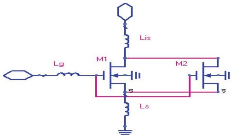
**Figure 8.** Structure of dual CS stage.
