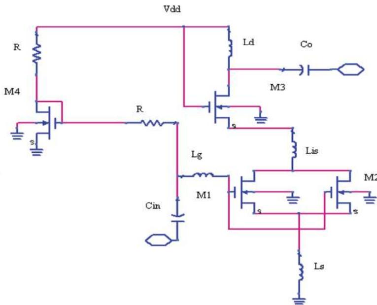
Figure 9. Schematic of SDC LNA.
