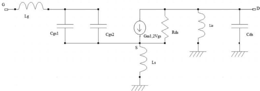
Figure 10. Equivalent model of input stage.
