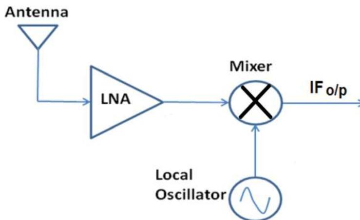
**Figure 3.** Block diagram of DCR front-end.
