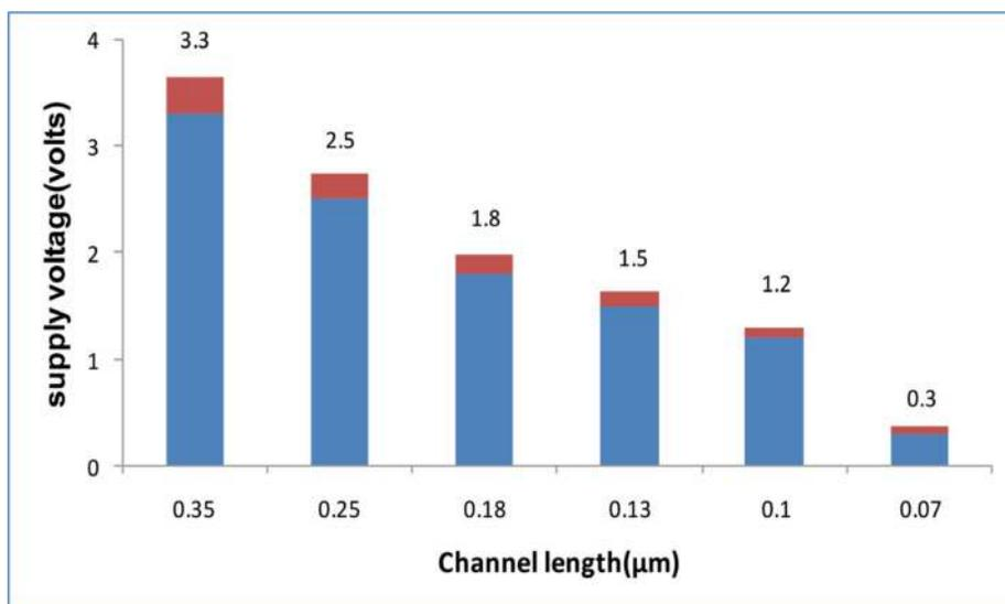
**Figure 5.** CMOS voltage scaling.
