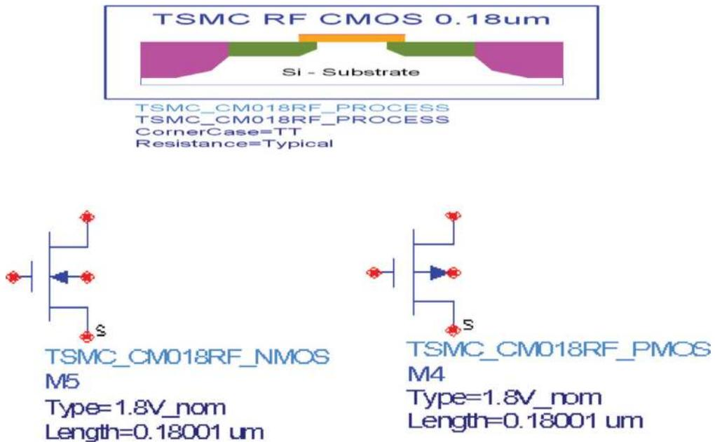
Figure 2. TSMC 0.18-μm RF CMOS models.
