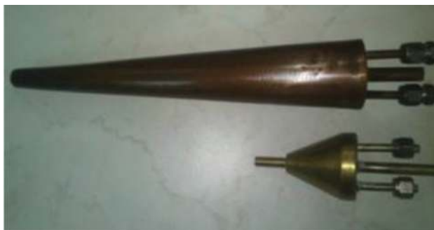
Figure 7. Photograph of the new and previous designed cold fingers.
