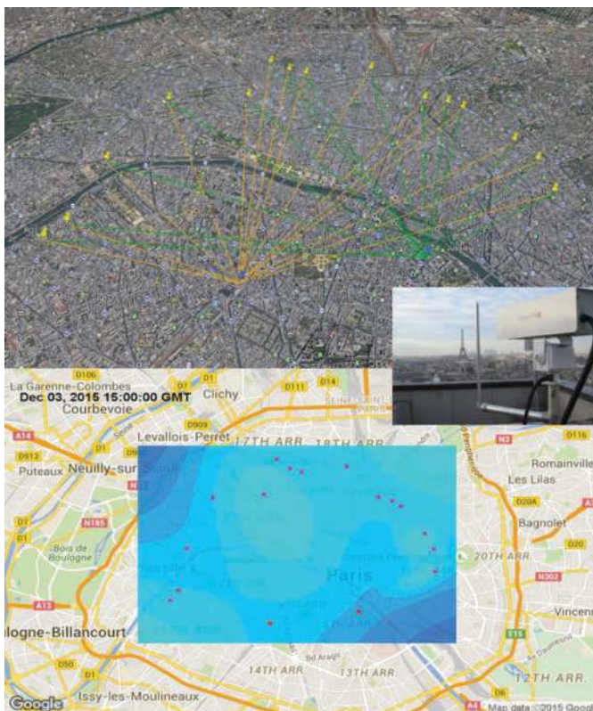
Figure 11. The disposition of transceivers and retroreflectors placed on top of buildings in Paris roughly arranged in a hemisphere. Orange and Green rays are chords, or paths, between a transceiver and one of the 15 retroreflectors. Images courtesy of J.T. Dobler, Spectral Sensor Solutions, LLC & T.S. Zaccheo, Atmospheric and Environmental Research.
