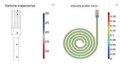
Figure 9. Particle distribution and velocity profile obtained in COMSOL Multiphysics<sup>®</sup>.
