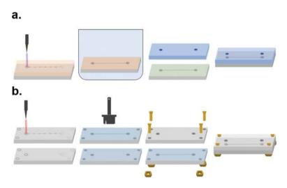
Figure 7. Manufacturing process of biomicrosystems. (a) Chemical etching process, and (b) laser engraving and cutting.
