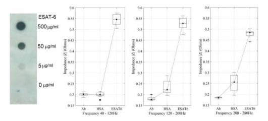
**Figure 5.** (a) Detection limit for the dot blot assay compared to the electro-immunosensor. (b, c, d) Analysis of impedance variation for 0.5  $\mu$ g/mL of analyte. (b) Impedance magnitude at 40–120 Hz, (c) impedance magnitude at 120–200 Hz, and (d) impedance magnitude at 200–280 Hz.
