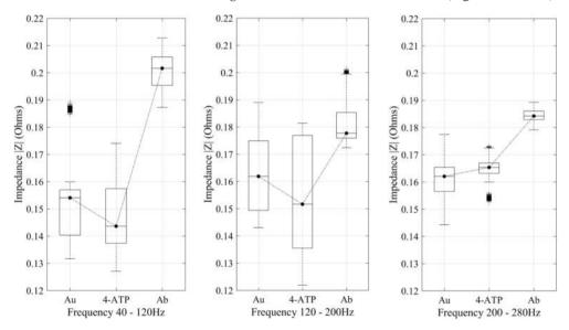
**Figure 4.** Analysis of impedance variation for the three main manufacturing stages. (a) Impedance magnitude at 40–120 Hz, (b) impedance magnitude at 120–200 Hz, and (c) impedance magnitude at 200–280 Hz.
