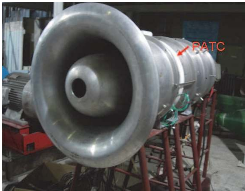
Fig. 29. Low speed axial compressor test rig with PATC
