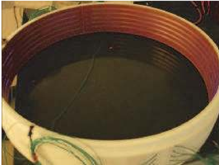
Fig. 28. Plasma actuation treated casing
