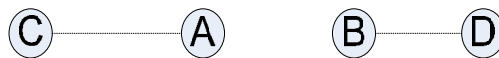
Fig. 1. S-MAC: Neighboring nodes A and B have different schedules. They synchronize with nodes C and D respectively
