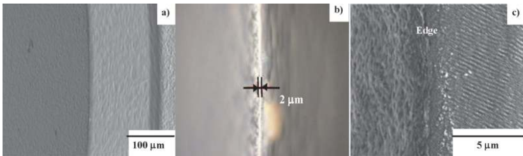
Figure 8. SEM and LM images on the laser treated side surface from the punch edge. (a) SEM image on the laser-trimmed head and side surfaces of punch in low magnification, (b) LM image around the punch edge, and (c) SEM image across the punch edge in high magnification. A nanostructure was formed to have a regular alignment with its period of 300 nm.
