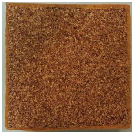
Figure 11. A sample of a 3-cm-thick corncob particleboard.
