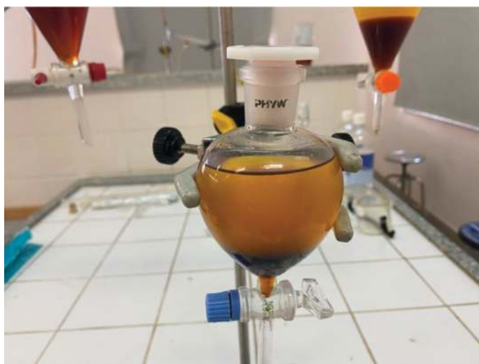
Figure 3. Decanting funnel installed at the bottom of the RD column.
