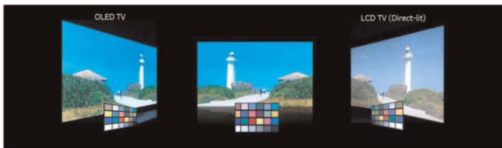
Figure 18. Picture quality change at the off-axis of the OLED TV and the LCD TVs.
