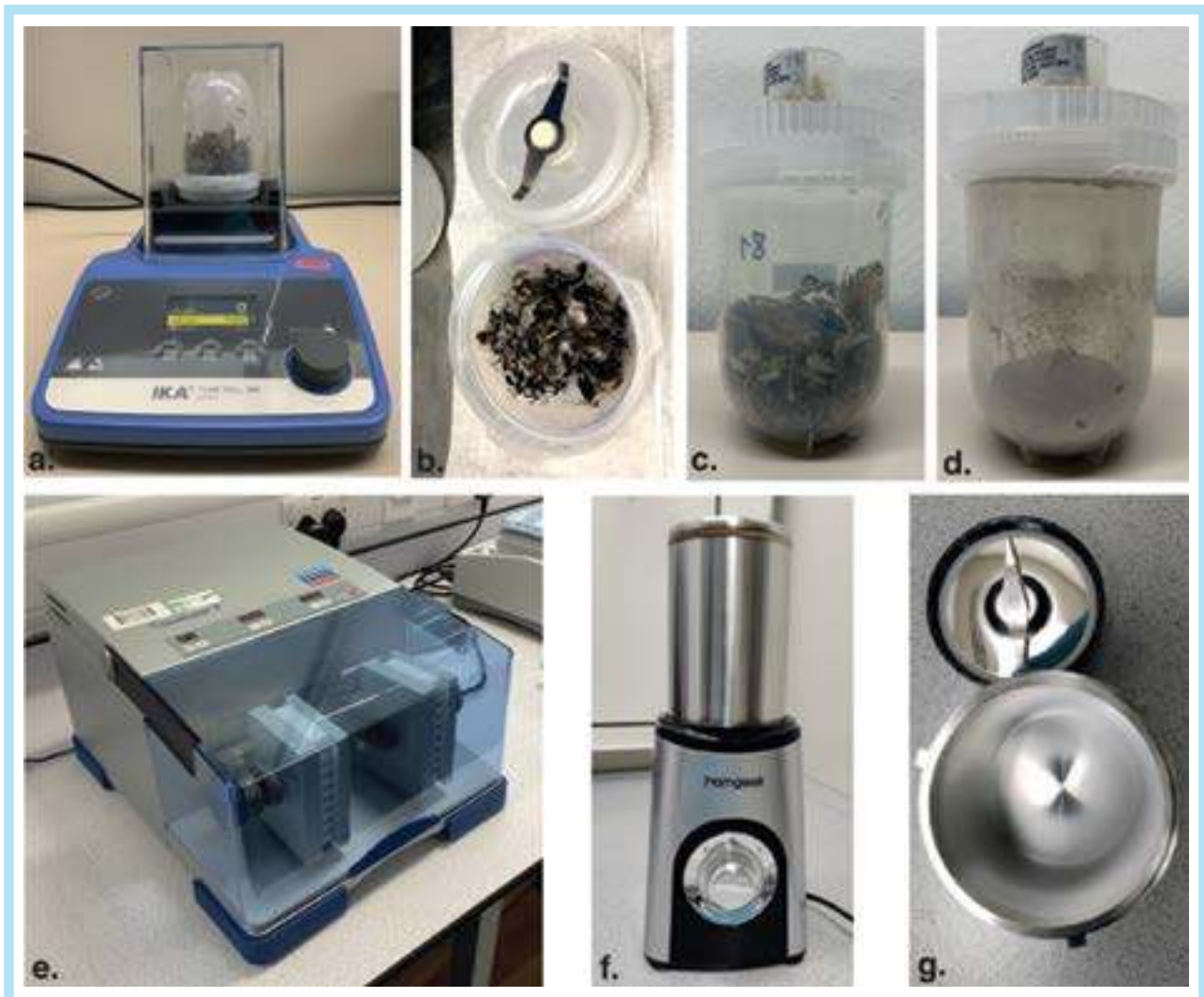
Figure 5. DNA homogenisation methods. DNA sample homogenisation protocols vary depending on equipment available, here we present a number of lab set-ups which show differing equipment for the homogenisation of tissue samples (dry and wet), IKA Tube-Mill 100 (a) with blending blades (b), dry malaise trap sample before and after homogenisation with the IKA Tube-Mill 100 (c and d), Qiagen TissueLyser II with plate attachment (bead mill also available) (e), and stainless steel wet-grinding blender (f and g).
