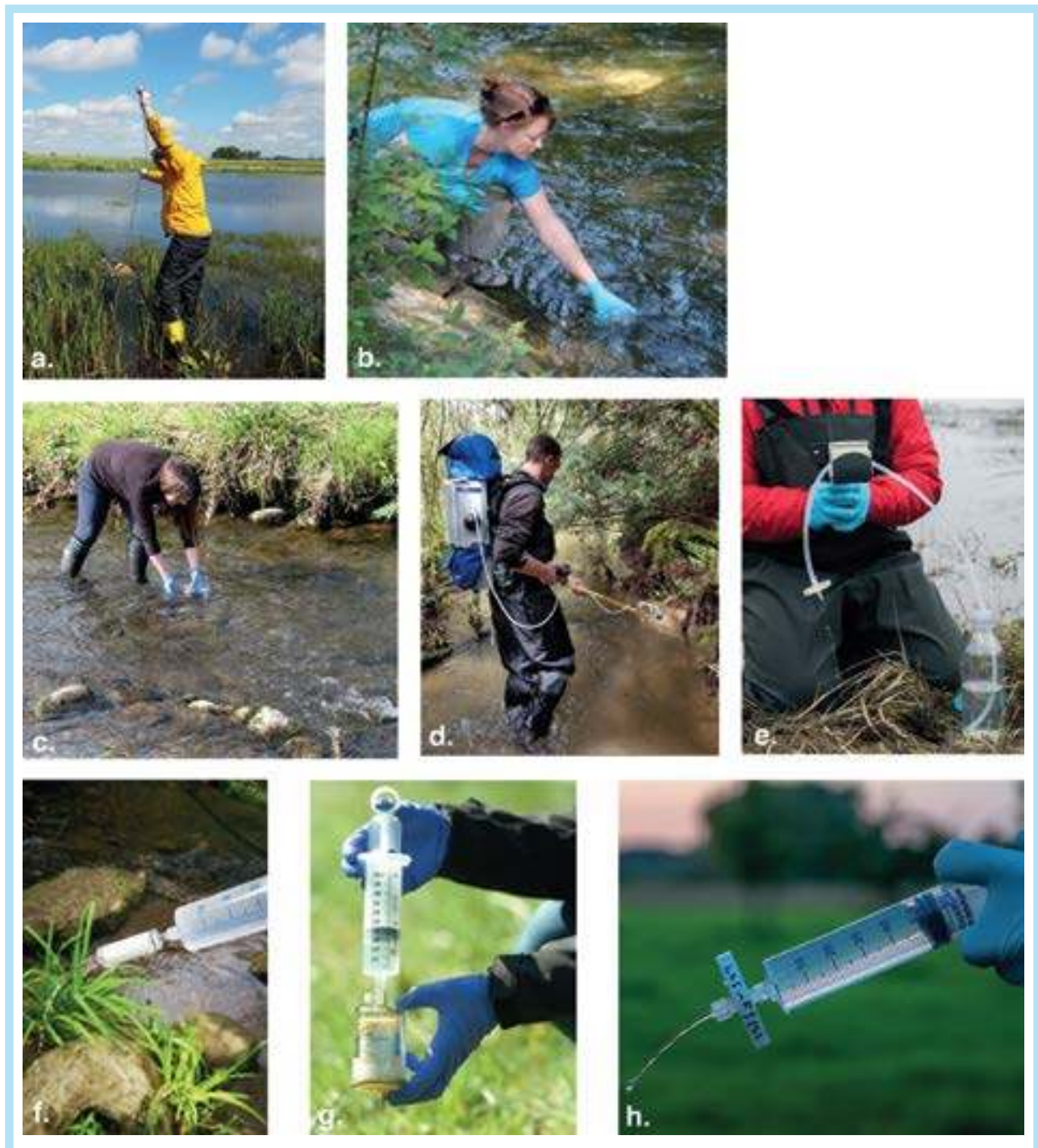
Figure 4. Water eDNA collection and filtration methods. Water collection should cause minimum disruption to the substrate of the water body, either by collecting the sample from the bank (a and b) without entering the water or by collecting the sample upstream of the sampler (c and d). Pairing filtration or sampling in the field with an enclosed filter is recommended to minimise potential contamination. Filtration in the field can be carried out with a peristaltic pump (e) or by using a disposable syringe (f, g and h).
