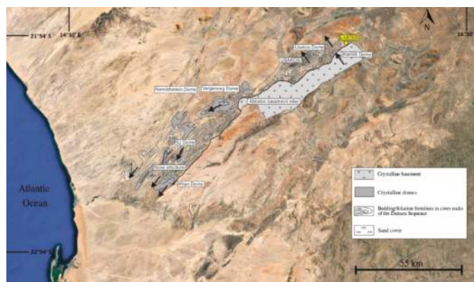
Figure 2. Schematic map showing the northeast trending dome structures covered by the geological map, by [40]. The gneisses and/or the Pan-African granitoids constitute the cores of the dome structures, whereas the surrounding supracrustals of the Damara sequence are draped around the domes. The solid black arrows indicate the tectonic transport direction for domes [41–44] and the Karibib district in the northeast. The yellow rectangle indicates the area where the marble quarries are located.
