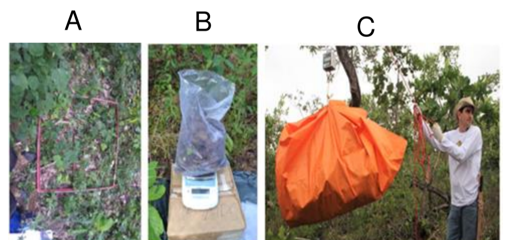
FIG 2. Fresh biomass measurement. A. Subplot quadrat for herbaceous layer. B. Field weighing with precision balance. C. Large volume weighing with dynamometer.
