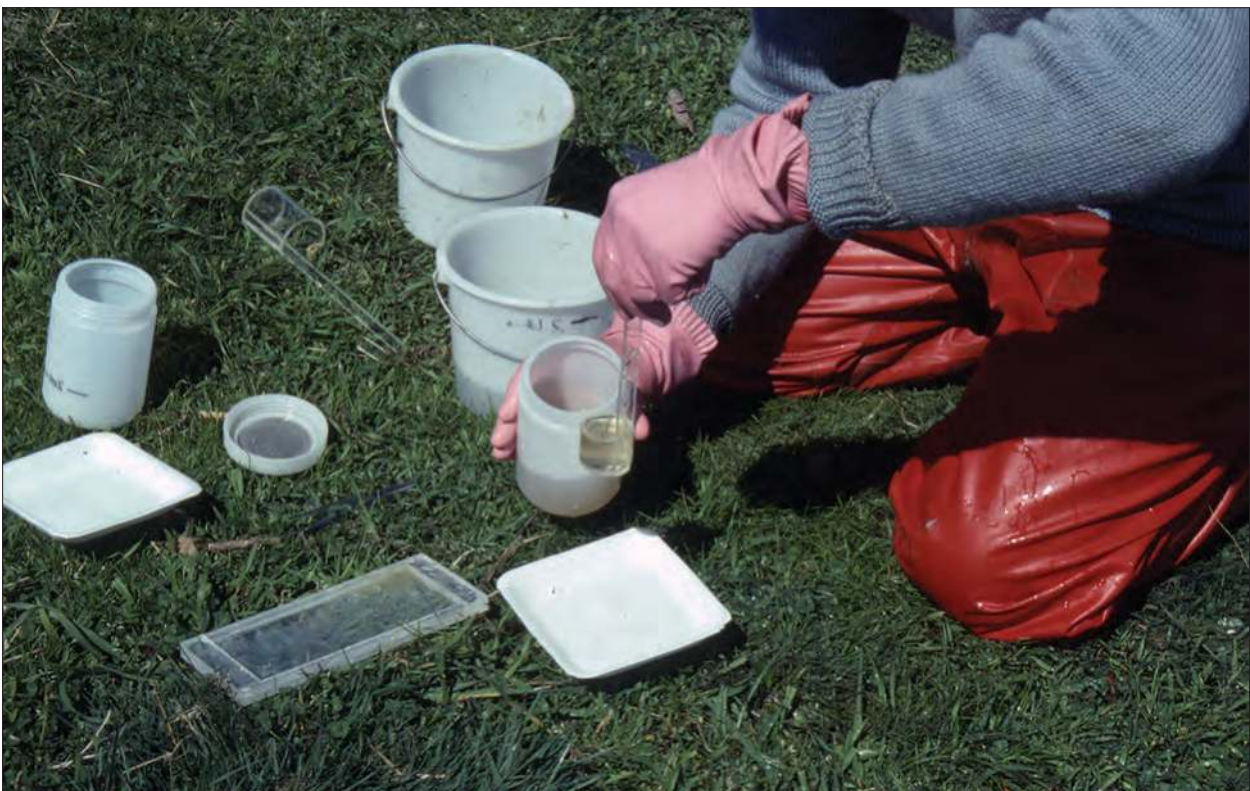
Figure 9.8: Two 20 mL aliquots are taken, placed into separate white polystyrene trays ready for staining. Photograph courtesy of KA Abbott.
