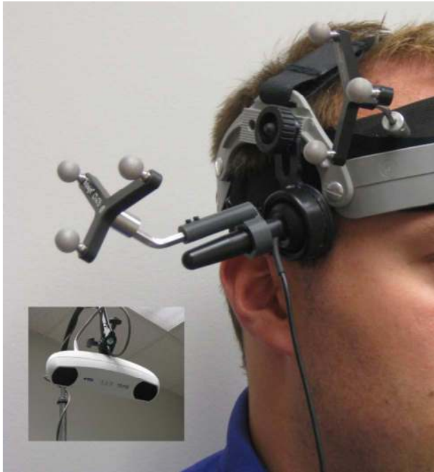
Fig. 2. Rigid bodies attached to example participant's head to track the three-dimensional position of the TCD probe relative to the participant's head. The rigid bodies are tracked by an infrared-emitting camera (inset; Polaris Vicra IR camera, Northern Digital Inc., Waterloo, ON, Canada) that emits IR light that reflects back to the camera by the passive IR markers fixed to each rigid body. Pictured is a TCD probe, a MARC 600 head mount (Spencer Technologies, Seattle, WA, USA) and rigid bodies (Brainsight, Rogue Research, Montreal, QC, Canada).
