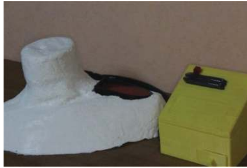
Figure 3. Acupuncture simulator model of GB21 (ASM21) equipped with a sensor detector light alarm.
