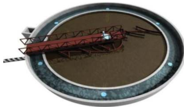
Figure 5. The thickener clarification of AMD water in the Sınak Coal Mine Site for fishery pool remediation e - .
