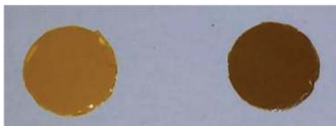
Figure 4. Photographs of pristine reference Kapton (left) and a radiation damaged Kapton sample (right) taken after an electron dose of 5.6 \times 10^7 Gy. Right picture was taken after 2 min of air exposure.
