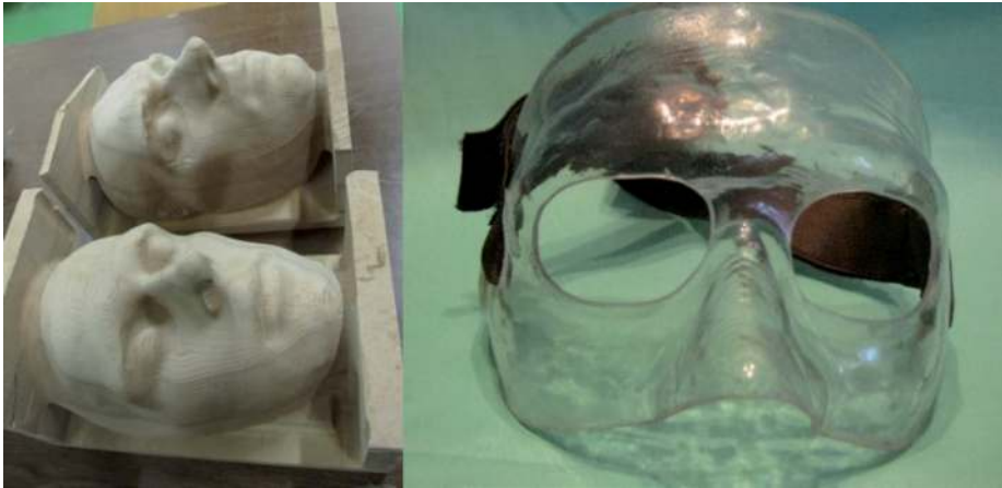
Figure 14. Molds made on three-axis milling machine and custom protective facial mask.
