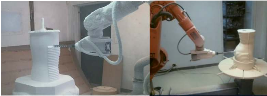
Figure 9. Robot-assisted spinal orthosis molds production.
