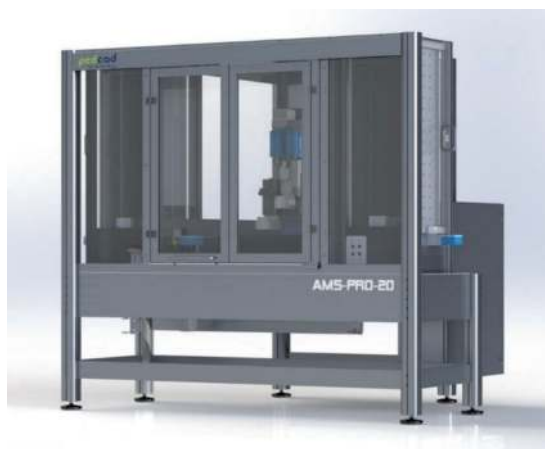
Figure 13. Modern three-axis milling machine for foot orthoses production (courtesy of PedCAD GmbH).
