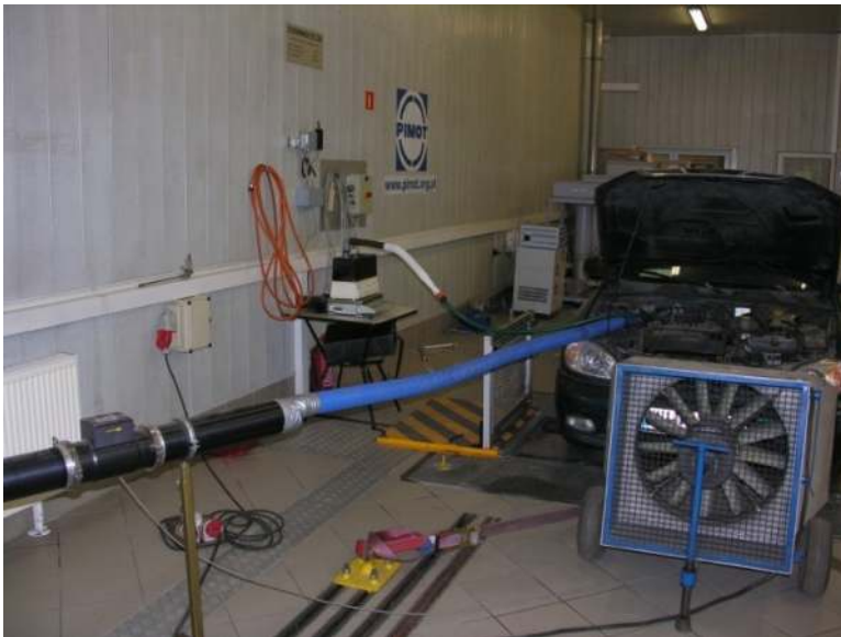
Figure 7. Photography of a test stand (visible chassis engine test stand, air supply, water vapor supply, and exhaust gas analyzer)
