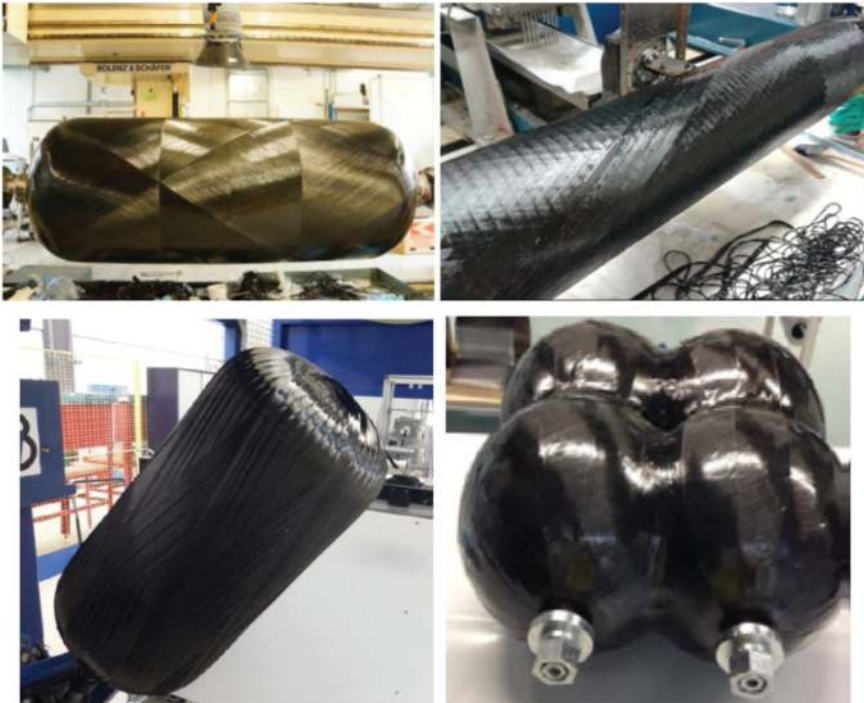
Figure 14. Four different composite tanks of CHATT project.
