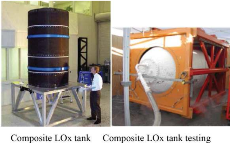
Figure 15. Composite lox tank of LM.
