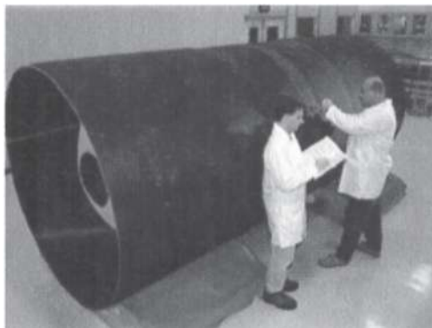
Figure 5. North Grumman's LH2 cryotank [15].
