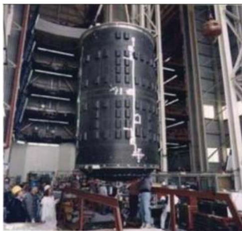
Figure 2. DC-XA composite LH2 cryotank.
