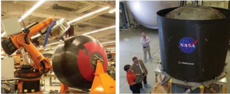
Figure 8. 2.4-m diameter tank, a robotic arm applies composite laminate [21, 22].
