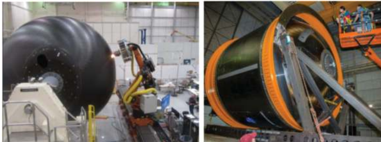
Figure 9. 5.5-m diameter tank [21, 22].
