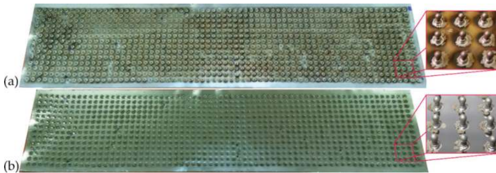
Figure 3. Example of metal sheet after pin deposition, where: (a) before; and (b) after cleaning.
