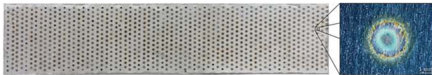
Figure 11. Example of the dark marks on the metal surface of the small-sized FMLP (MPin-C-MPin hexagonal 5 mm with dimensions \approx 350 \times 80 \times 4 \text{ mm} ) caused by pin deposition process.
