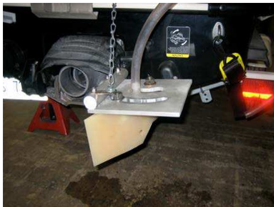
Fig. 8. The custom-designed center-point swivel and ram intake for the YSI PSK.
