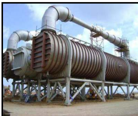
(a) Circular vessel evaporator.
